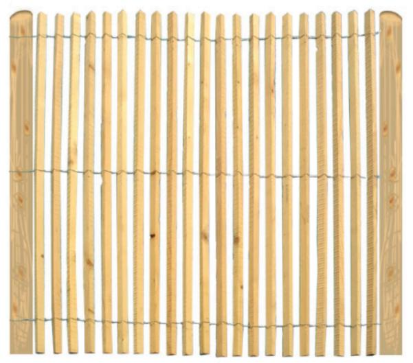
This is one wing of a sand fence section. A section consists of 6 wings wired to a center post and anchored on each end by a post. The wings are 4 feet by 4 feet. The posts are 3 inches in diameter and are 8 feet long. The posts are placed in the ground 4 feet.
