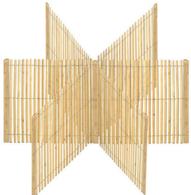
This structure consists of six 4 foot by 4 foot wings wired to a common center post and anchored on each end by a single post. Thus, one section consists of 6 wings and 7 posts.
