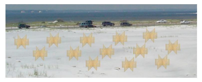
The installation pattern is based on the eight foot diameter (2.5m) of each section. These are spaced along a line at eight foot intervals leaving an eight foot gap between each section. A second row is then added to place a section in front of the gap created by the previous row. This pattern is continued until the area needing sand dune formation is covered with sections. Two rows are required as a minimum.
