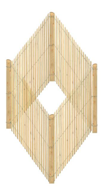
This design allows installation within a zone where marine sea life, such as turtles and shorebirds may be active. Because the configuration is diamond shaped with the long axis aligned with the landward-seaward line (perpendicular to the shore), animals moving along that path would be diverted in a diagonal direction along the perimeter of the section. Because the section is closed, no dead-end entrapment is possible.
